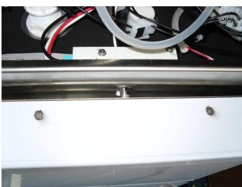
6) Check if the door is hard during the closing. This matter is caused by wrong adjustment of door, which is making friction with the door gasket in the lower part of chamber. To solve this problem it needs to unscrew the door hinges and move the door up a little bit.
