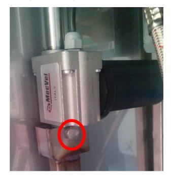
Remove the actuator from the brassk block unscrewing the yellow highlighted screw
