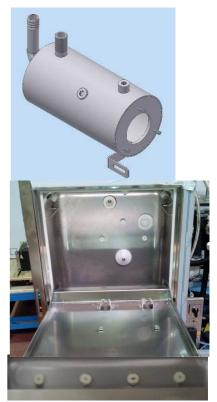
Check if the one way valve is covered in limescale. If that's the case, leave it for some time in a solution of water+softener and rinse thoroughly (ACTION 61).
