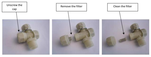
Extract the cylindrical filter inside the cap, clean it thoroughly (possibly using compressed air).
