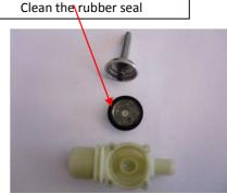
Place the pieces in their seat and tighten the 4 screws all the way down (warning: mount the metal plate positioning the slot facing the seal holder).
