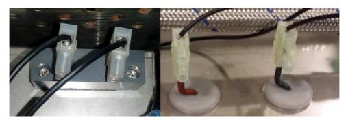
Disconnect the connectors (please be careful remembering the way they're connected to the probes) and check the conditions of the probes themselves.
