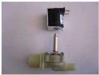
Loosen the metal hose clamps and remove the solenoid valve by unscrewing the plastic ring located on it.
