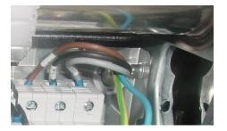
7. The first component to be replaced (or adapted by cutting the unused wires) is the power cable.
