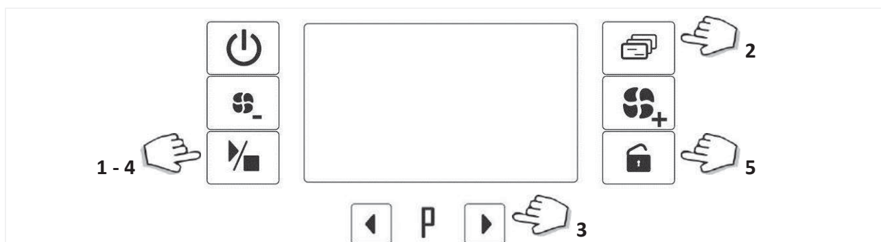
fig. 28 – Steps for display and modification of the Set and Cloc parameters: Access the parameter: by pressing the Start/Stop button Quit the parameter: by pressing the Door opening button.
