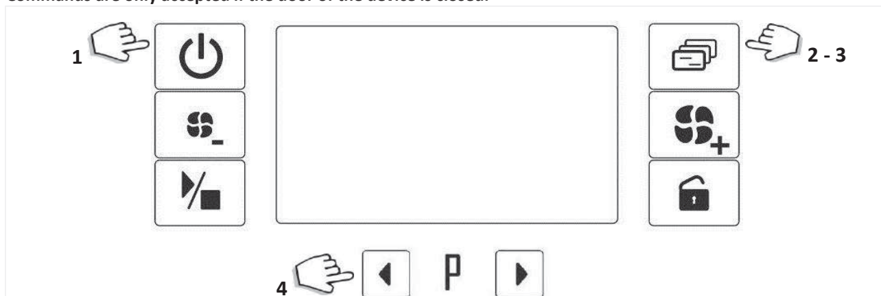
fig. 26 – Standard procedure for forcing printing. Last cycle data: use “On/Off”+“Functions” keys; Parameters: use “Functions”+“LH Selection” keys.
